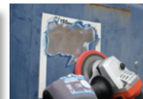
After 12.77 seconds of grinding
